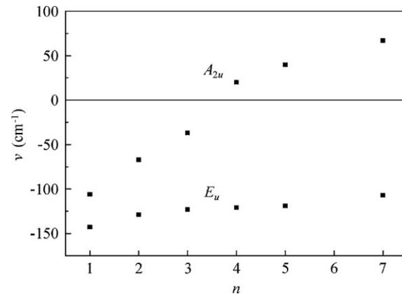
**Figure 1** Frequencies of lowest  $A_{2u}$  and  $E_u$  polar optical modes in the paraelectric  $P4/mmm$  phase as a function of the thickness of the KTaO<sub>3</sub> layer in (KNbO<sub>3</sub>)<sub>1</sub>(KTaO<sub>3</sub>)<sub>n</sub> superlattices. Imaginary frequencies of unstable modes are plotted as negative values.
